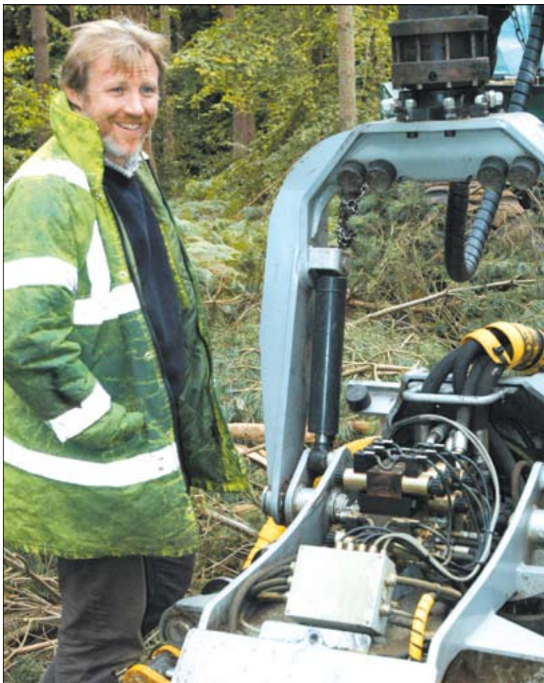
Access to the hydraulics on the 30RHS is excellent.
