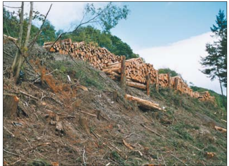
One of the first requirements had been maximising the capacity of the restricted timber landing area. Trees on the roadside edge had been cut high to safely support the stacks above the steep bankside.
