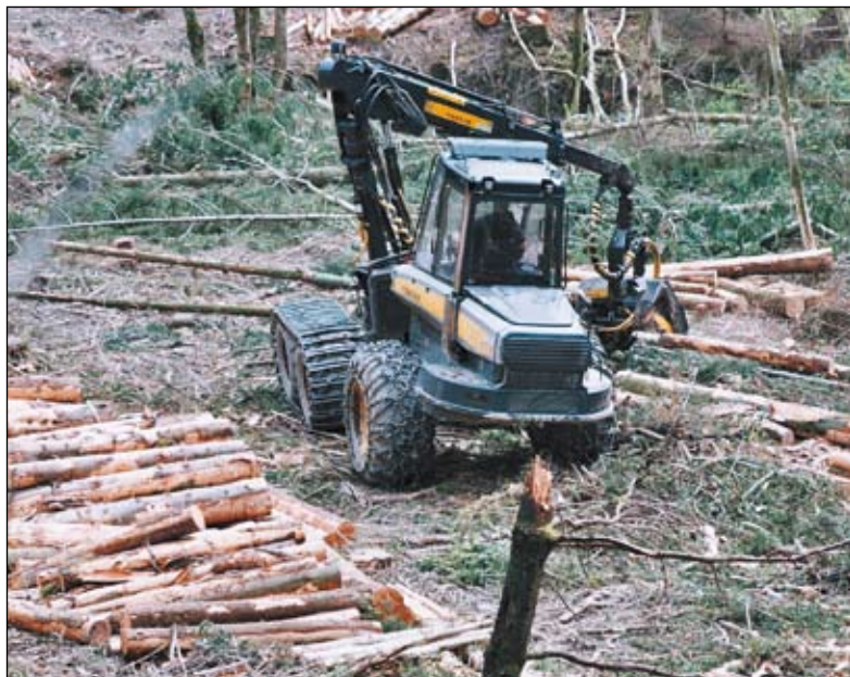
Gareth Davies aboard the Ponsse Ergo harvester processes timber felled by chainsaw on the far side of the watercourse that runs through the harvesting site. The felling capability of the Ergo was used where possible, but this still left many stems to be felled by the chainsaw.
