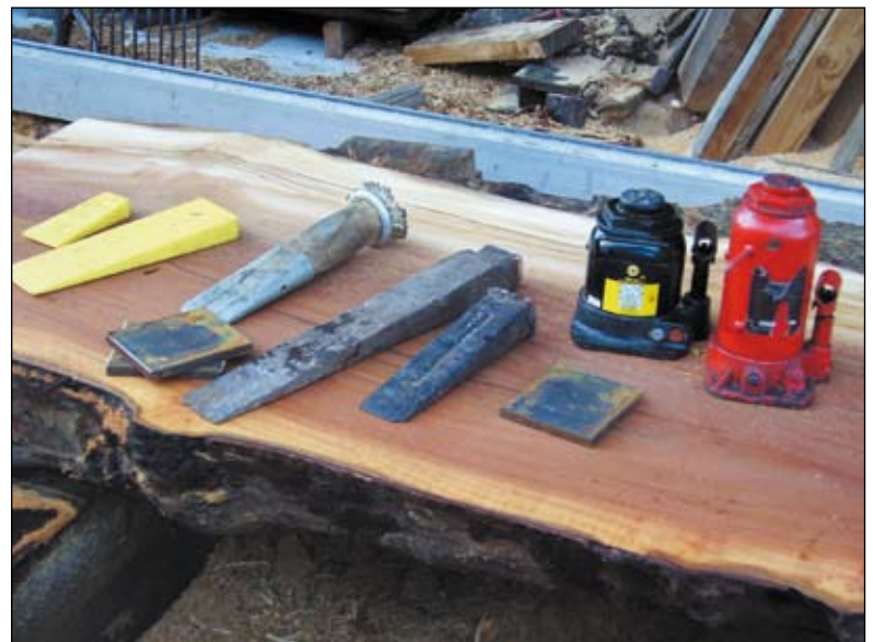
(Left) The downed tree, with a little too much hinge wood left in the centre due to too short a chainsaw bar. (Right) Tools of the trade (left to right) plastic wedges, alloy Highlift wedge, steel plates for use with the steel wedges, a jack plate, a heavy duty low-profile jack, and a normal height jack.
