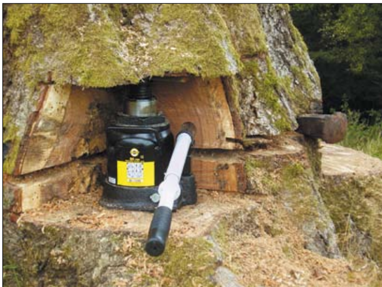
(Left) The jack is already set into the jack-seat alongside the safety wedge, but the timber above the jack is beginning to buckle. (Right) A new jack-seat has now been cut into the trimmed butt.
