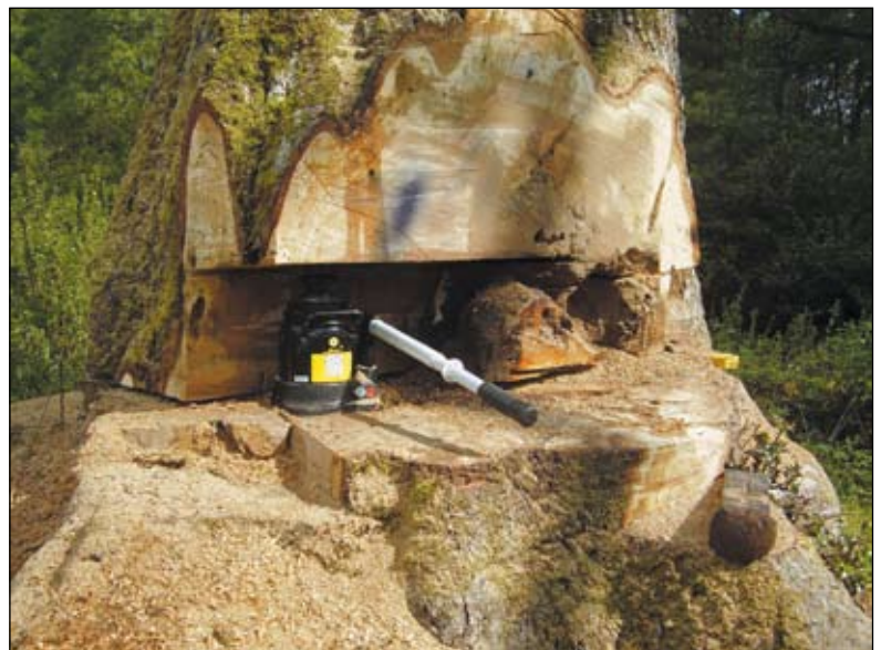
(Left) The jack is already set into the jack-seat alongside the safety wedge, but the timber above the jack is beginning to buckle. (Right) A new jack-seat has now been cut into the trimmed butt.
