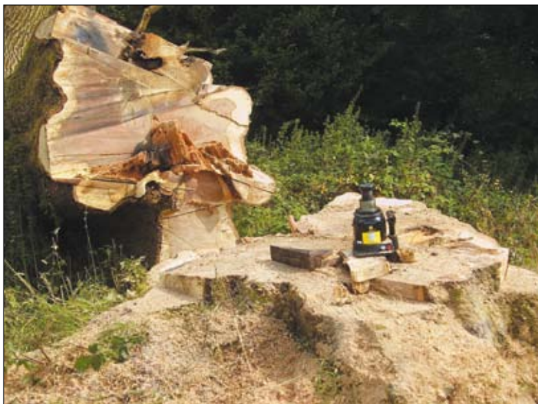
(Left) The downed tree, with a little too much hinge wood left in the centre due to too short a chainsaw bar. (Right) Tools of the trade (left to right) plastic wedges, alloy Highlift wedge, steel plates for use with the steel wedges, a jack plate, a heavy duty low-profile jack, and a normal height jack.
