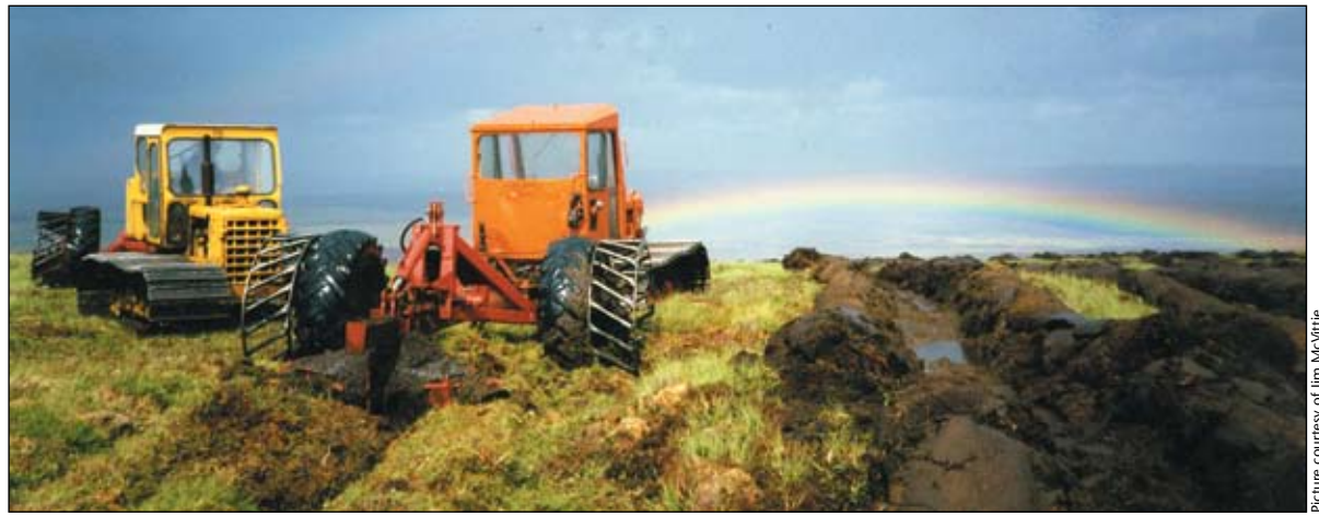
Clark trailed single-furrow ploughs with double throw moldboards, fitted with cage wheels, belonging to Dalgleish Brothers of Moffat.
