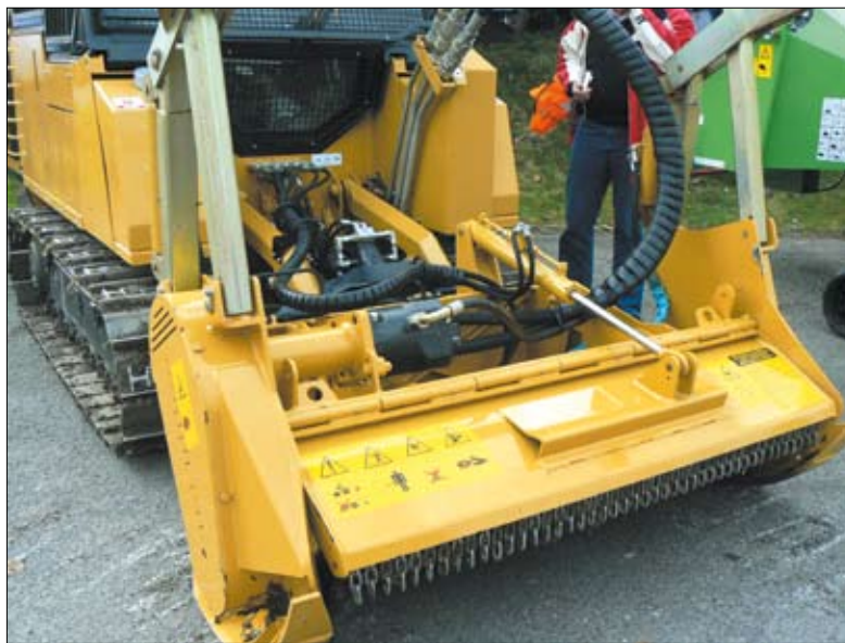
(Left) Back at base and an opportunity to get to the guts of the Multi-Task 120. (Right) View of the heavy-duty mulching head and the quick hitch system for mounting a range of tools.
