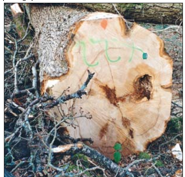
(Left) This may not look good to the untutored eye, but the defects in this butt are age cracks that often appear after large oaks are felled. One solution in a butt this size is to ‘quarter saw’ along the line of the major cracks and resaw along the grain. This would produce panels with beautiful wide silver banding, such as were used in the interior of the Palace of Westminster. (Right): This tree promised to be one of the best in the Touch Estate parcel but the buyer was to be desperately disappointed. What can be salvaged will probably be destined for ‘fencing oak’. The cavity would be a small problem but the cracks crossing the log are ‘star shake’. The dark stains have been in the tree for years and continue to the top. The dark circular stains show the presence of ‘ring shake’.
