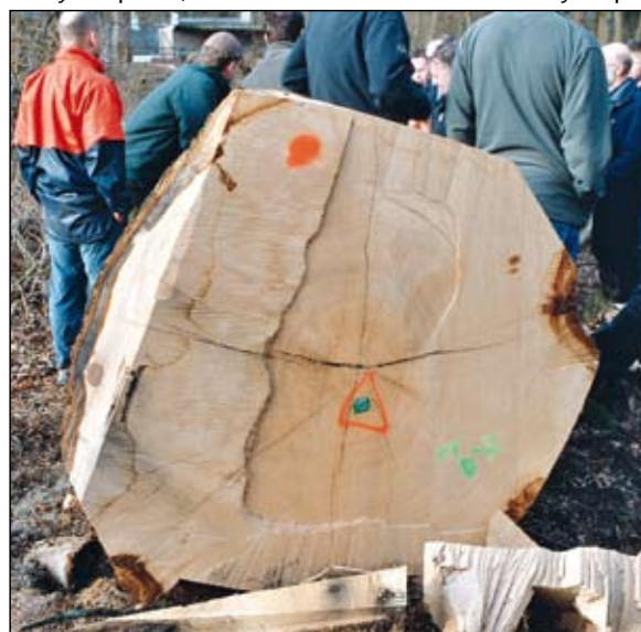
(Left) This may not look good to the untutored eye, but the defects in this butt are age cracks that often appear after large oaks are felled. One solution in a butt this size is to ‘quarter saw’ along the line of the major cracks and resaw along the grain. This would produce panels with beautiful wide silver banding, such as were used in the interior of the Palace of Westminster. (Right): This tree promised to be one of the best in the Touch Estate parcel but the buyer was to be desperately disappointed. What can be salvaged will probably be destined for ‘fencing oak’. The cavity would be a small problem but the cracks crossing the log are ‘star shake’. The dark stains have been in the tree for years and continue to the top. The dark circular stains show the presence of ‘ring shake’.
