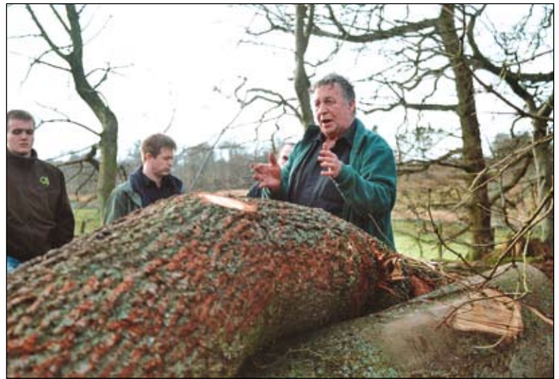
If the bend is right, oak can be saleable for boatbuilding or green oak construction. This limb looks good according to Gavin Munro. A small limb is often found to have grown at the apex of the bend, as it has here, but if the knot is still alive it should be acceptable.
