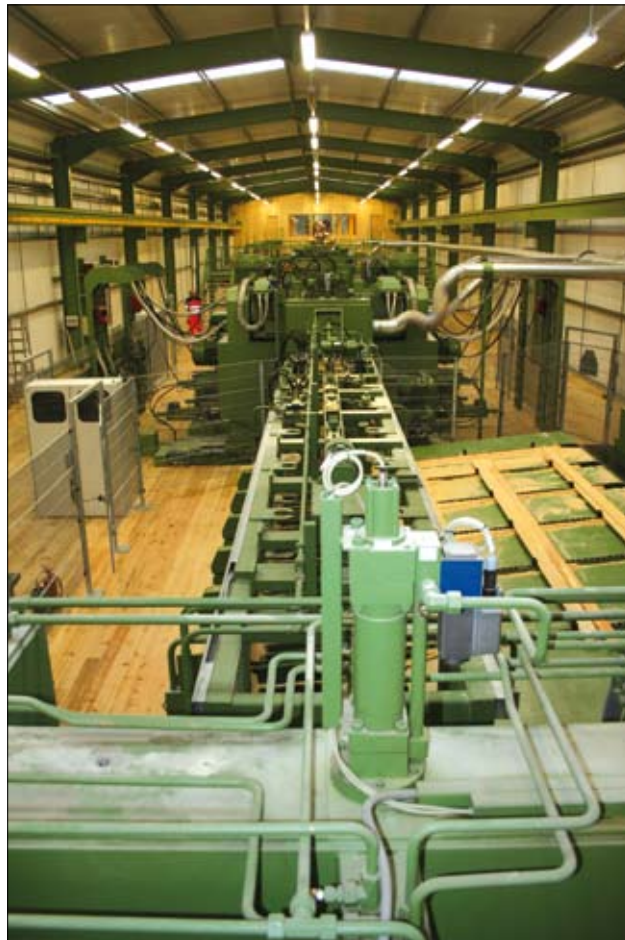
(Left) General view of part of the opening section of the line. (Top) The first thing that happens to a log as it enters the mill is that it is turned the right way up to maximise recovery. (Above) After the canting process, the log sets off towards the profiler.
