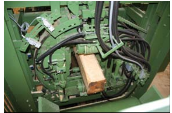
(Left) General view of part of the opening section of the line. (Top) The first thing that happens to a log as it enters the mill is that it is turned the right way up to maximise recovery. (Above) After the canting process, the log sets off towards the profiler.
