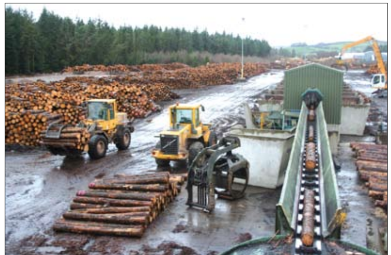
Logs being selected, scanned and sorted on the log line. The new scanners are housed in the green hut.
