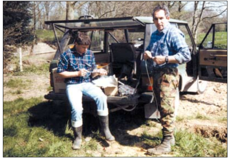
Bob Eames (right) with John Cooper's son Christopher, twenty years ago, drilling holes in sticks of gelnignite ready to feed white plastic instantaneous fuse through them.
