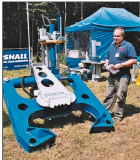
(Left) Allan Marshall with Binderbergers great and small. The Herkules crane-mounted grapple splitter (foreground) is available in 30 and 40 tonne versions. (Right) The German manufacturer of BGU machines expects them to be taking a bigger share of the British market in future. The SP30 is the most powerful BGU log splitter.
