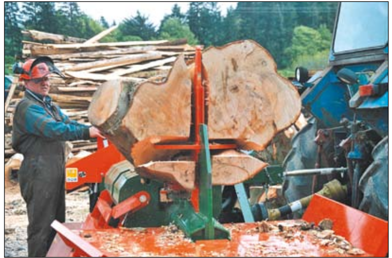
A Posch SplitMaster makes the first pass through a knotty lump of beech. The height of the splitting knife can be raised and lowered hydraulically.
