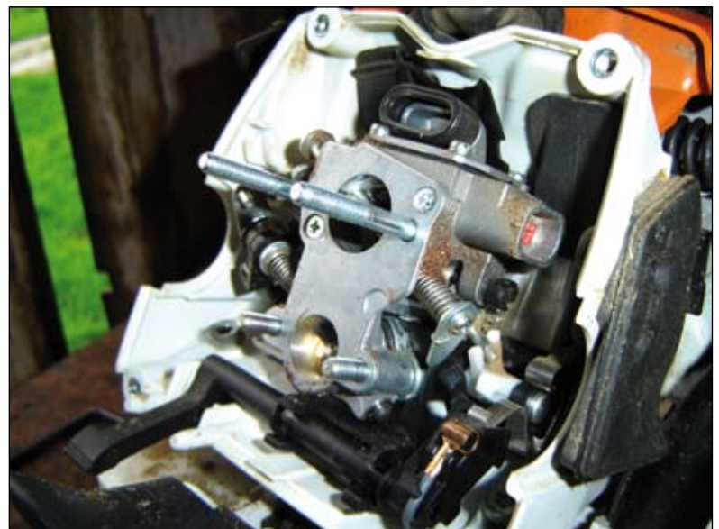
(Left) The complex carburettor is an integral part of the new stratified scavenging design. (Right) Red plugs in the air screw holes mean there's no tuning this demo saw!
