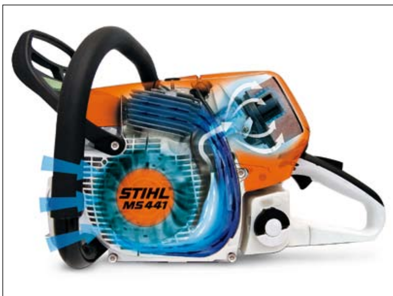
(Left) Schematic showing how the centrifugal air cleaning system, which is new to Stihl, should work. The dirt sticking to the inside of the cover in the picture on the right shows that it does.
