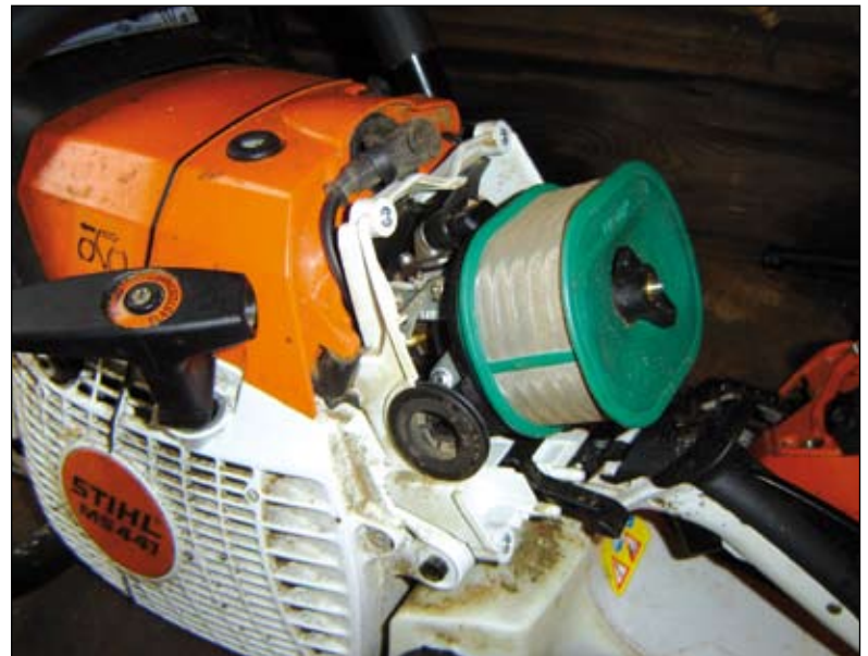
At last a sensible air filter, and after many hours of work it is still fairly clean.
