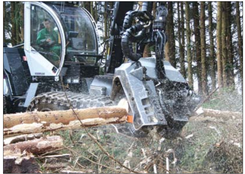
(Left) The 8H harvester is fitted with a Loglift 220 10 metre parallel crane. (Right) The new 8L head.
