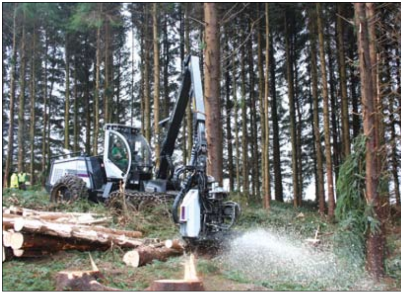
(Left) The 8H harvester is fitted with a Loglift 220 10 metre parallel crane. (Right) The new 8L head.
