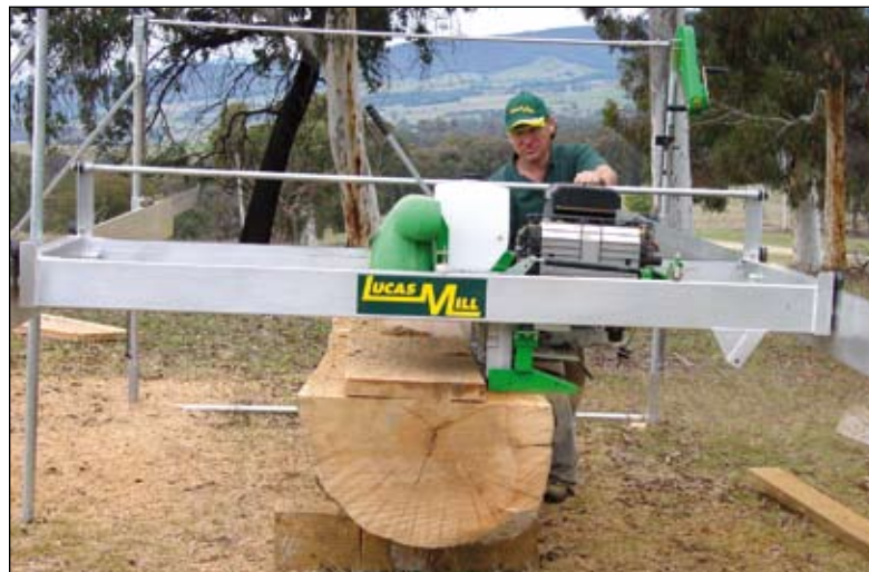
(Left) You can't get more portable: the Alaskan chainsaw mill from Granberg, cutting lime. (Above) Fuelwood Harvesting's Australian made Lucas Mill.
