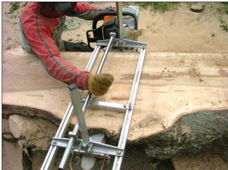
(Left) You can't get more portable: the Alaskan chainsaw mill from Granberg, cutting lime. (Above) Fuelwood Harvesting's Australian made Lucas Mill.
