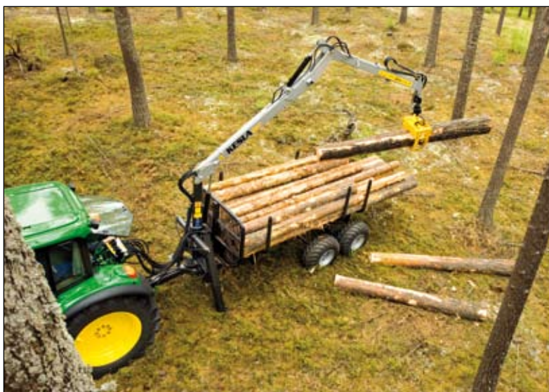
Kesla 8T trailer with 202T loader which has a 1.2 metre boom extension.
