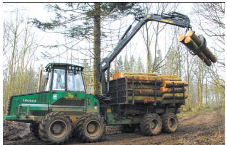
There are around ten tonnes of saw logs on the Logset forwarder. John bought these machines – the Logset 506H harvester and 6F forwarder – brand new in 1999. Because he has spent so much on maintenance they have a lot of life left in them, and because they are 'paid for', the pressure is off. He would not want to have to put them on front-line work – they are better on private estates.
