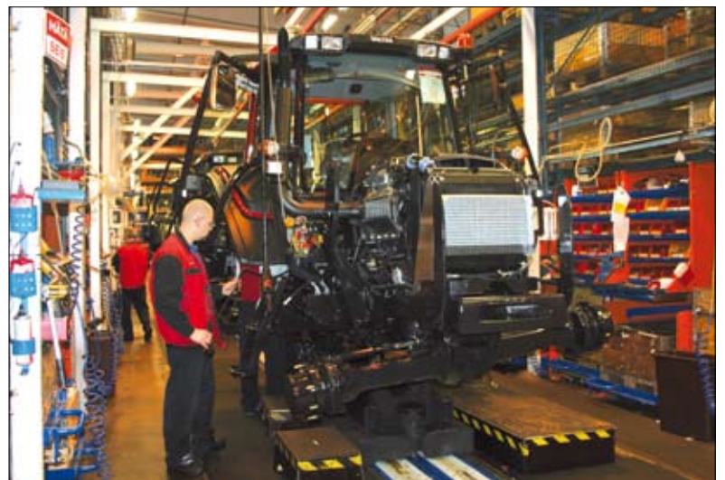
(Left) Can you tell what it is yet? The drive line will be connected to the middle frame before passing along the assembly line (right). Some 50 tractors make this journey every working day.
