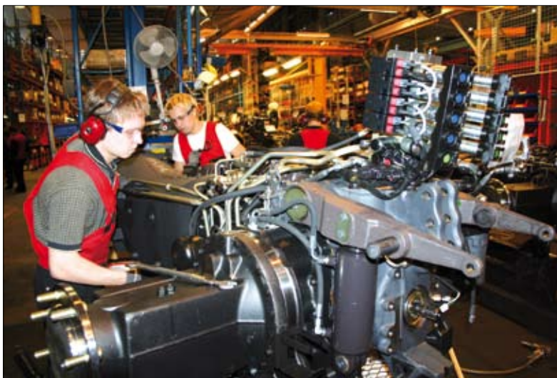
(Left) Can you tell what it is yet? The drive line will be connected to the middle frame before passing along the assembly line (right). Some 50 tractors make this journey every working day.
