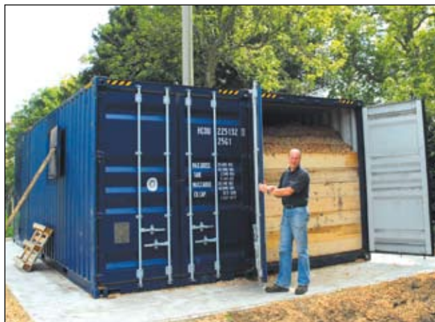
(Left) The Valtra 8150 140hp tractor tows the Heizohack HM 8 400 PTO powered trailer mounted chipper. It has 8 knives and a 400 mm aperture. The chipper was bought for £22,000 + VAT and delivered in June 2007. (Right) Toby Askew stands by the chip store. A trench has been dug below the store so that the chipper can feed chip straight into the store.
