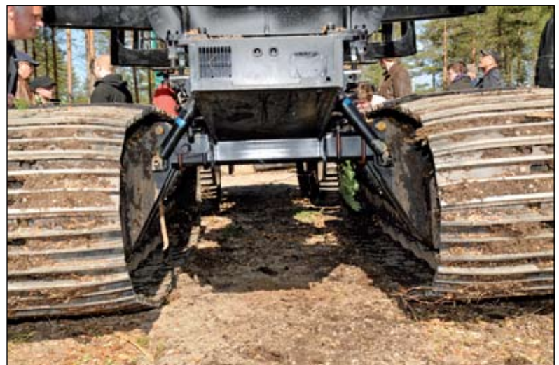
Each track is attached to the framework/chassis with two springs and a shock absorber. This gives a gentle ride which is kind to the terrain. The springs and shock absorber can be adjusted for various ground conditions.
