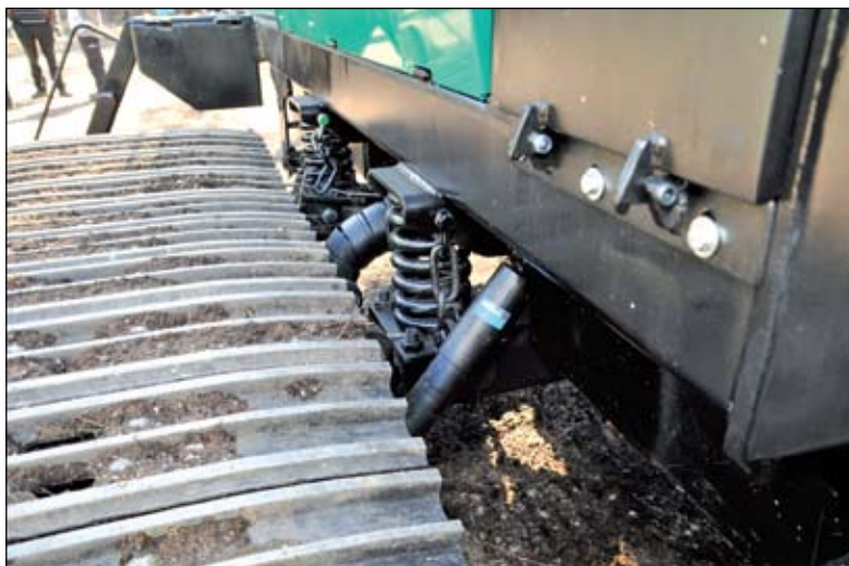
Each track is attached to the framework/chassis with two springs and a shock absorber. This gives a gentle ride which is kind to the terrain. The springs and shock absorber can be adjusted for various ground conditions.
