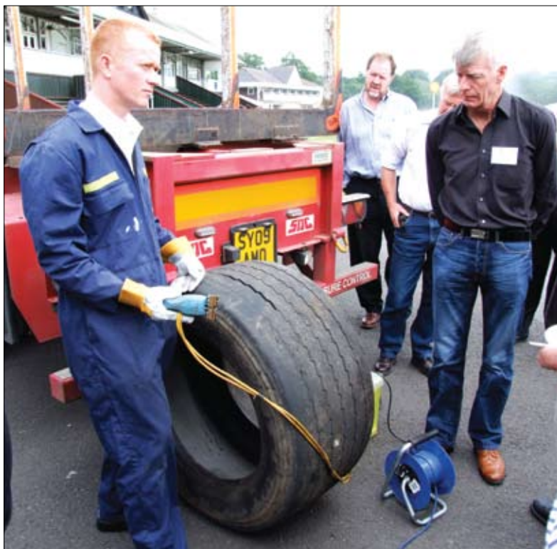
Michelin's tyre regrooving process being demonstrated in the car park during the lunch break.
