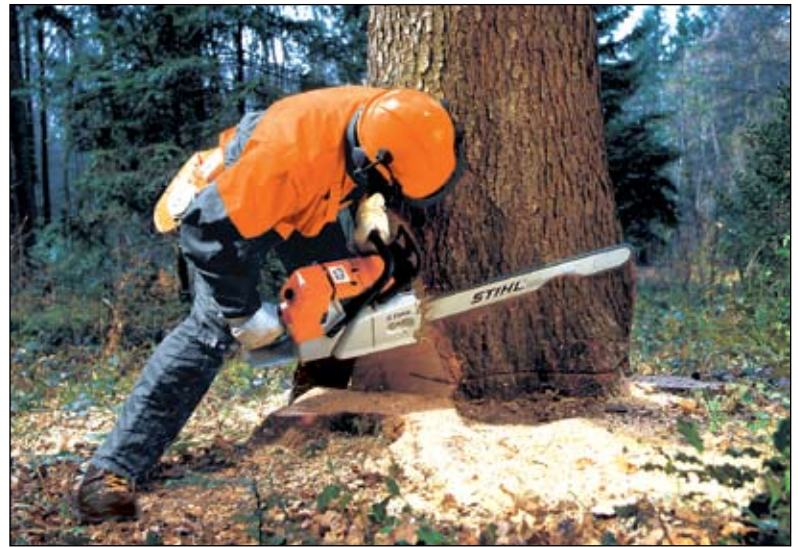
The heavyweight MS880 from Stihl, largest in their range at almost 122cc.
