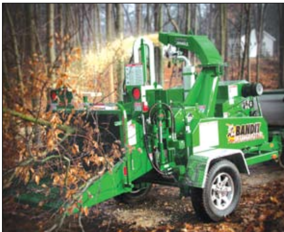
(Left) New from Bandit, the 990XP, 12" capacity, is a compact chipper with a 24" diameter drum. Engine options up to 86hp are available. (Centre) The DH series from Doppstadt is also available on tracks. (Right) The top of the range C1175 drum chipper from Europe Recycling.
