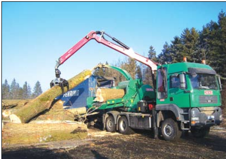
(Left) Jenz Chippertrucks are highly manoeuvrable and offer low transport costs. The 480hp MAN diesel powers both the chipper and the truck. (Right) The Junkkari HJ500 is operated via an electro-hydraulic remote control.
