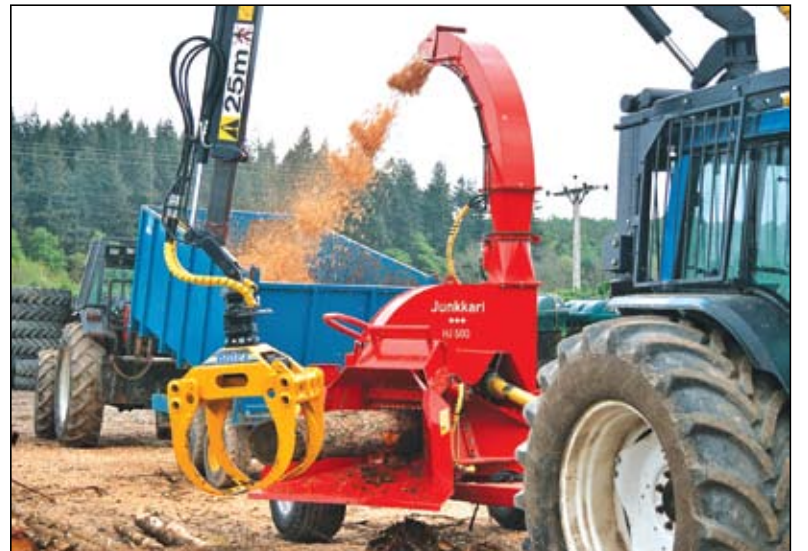
(Left) Jenz Chippertrucks are highly manoeuvrable and offer low transport costs. The 480hp MAN diesel powers both the chipper and the truck. (Right) The Junkkari HJ500 is operated via an electro-hydraulic remote control.
