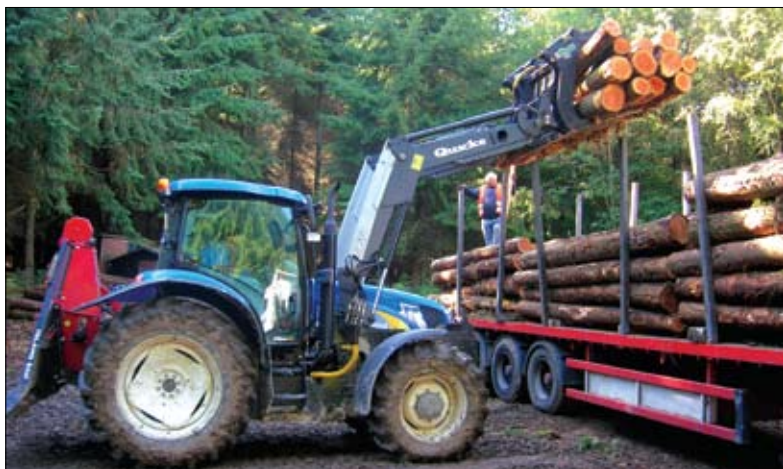
(Left) New Holland T6030 with Albutt grab loading small Douglas sawlogs. (Right) 60-year-old Douglas fir logs, which were extracted by skidder.
