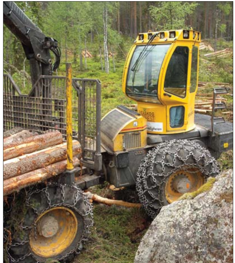
Self-levelling rotating cab, no bogies, and a 30kW electric motor turning each wheel.
