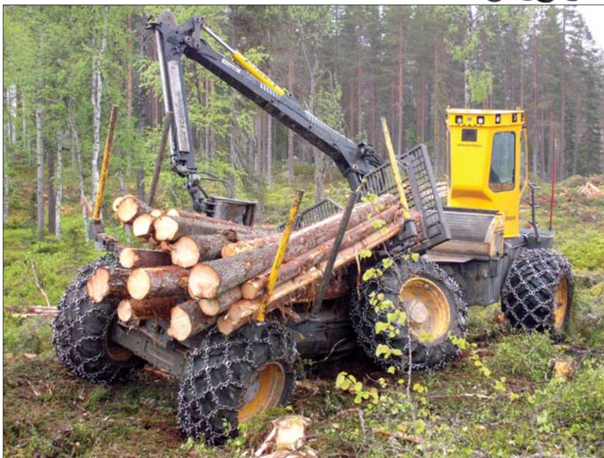
Your flexible friend, being tested to the limit by Calum Reid! The F14 has two centre joints, and it became clear that the centrally split rear trailer was using the logs almost as torsion bars to prevent turnover of either rear axle.
