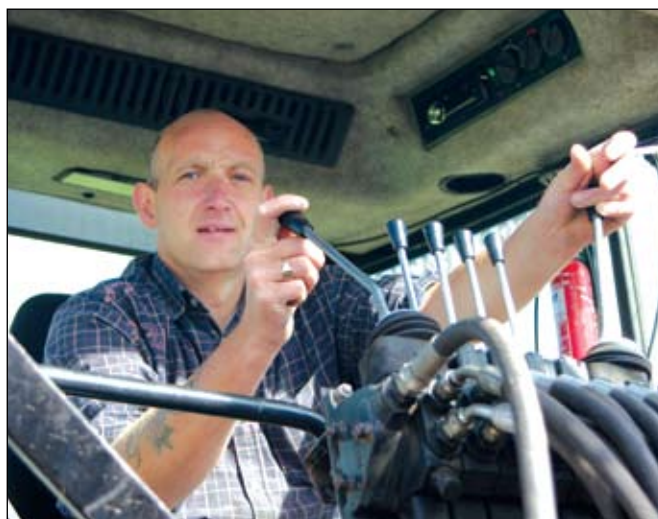
Rendered paraplegic as a young man, John McLeod was determined to return to hands-on forestry. However, it took some considerable time before this was possible. Thanks to the addition of a harness and hoist, he can manoeuvre himself in and out of the tractor's cab. The controls of his forestry tractor modified, John uses a hand-held command system to control the process, and now extracts timber sourced from his own harvesting contracts for use by his firewood processing business, Elm Tree Products.
