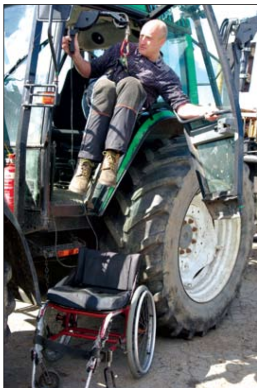
Rendered paraplegic as a young man, John McLeod was determined to return to hands-on forestry. However, it took some considerable time before this was possible. Thanks to the addition of a harness and hoist, he can manoeuvre himself in and out of the tractor's cab. The controls of his forestry tractor modified, John uses a hand-held command system to control the process, and now extracts timber sourced from his own harvesting contracts for use by his firewood processing business, Elm Tree Products.
