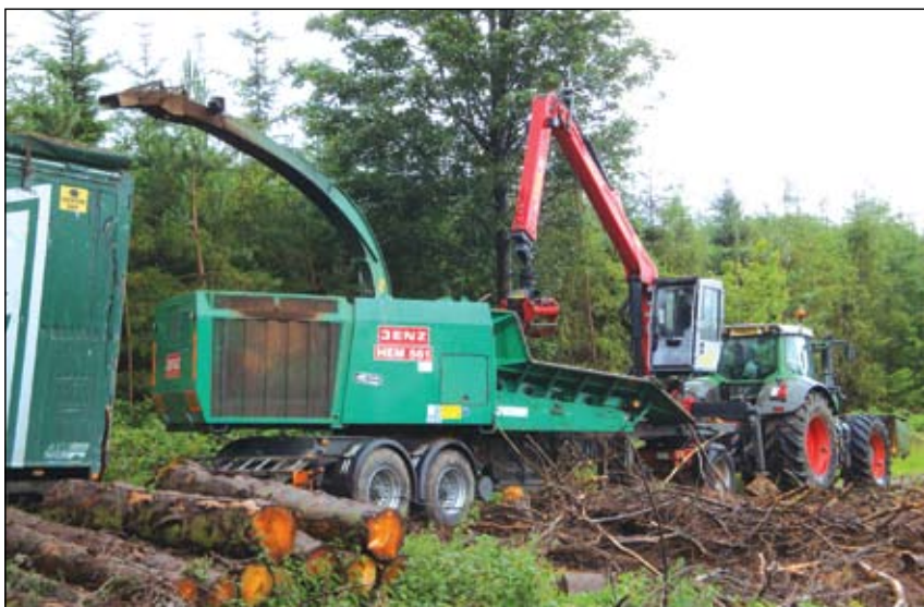
(Left) The Jenz Hem 561 chipping some of the 160 tonnes of brash brought to rideside. (Right) All estate machinery is shared between the farm and forestry departments. This Manitou MLT 634 LSU Turbo is used to load logs and lift the heavier pieces of timber and brash.
