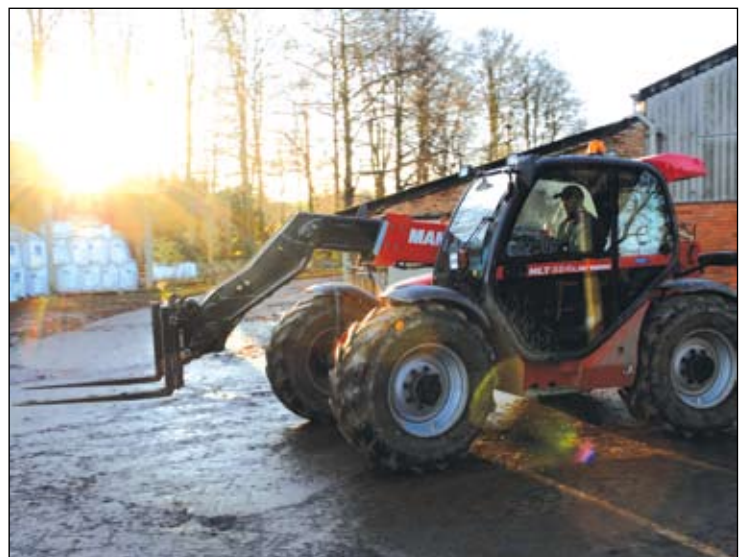
(Left) The Jenz Hem 561 chipping some of the 160 tonnes of brash brought to rideside. (Right) All estate machinery is shared between the farm and forestry departments. This Manitou MLT 634 LSU Turbo is used to load logs and lift the heavier pieces of timber and brash.
