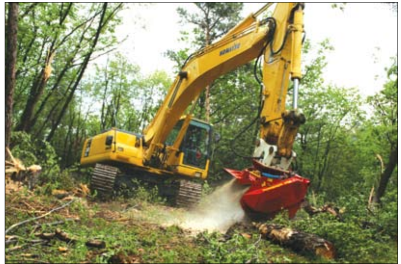
Seppi's Star FC, capable of mulching, stumpgrinding and stone crushing.
