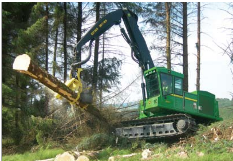
John Deere 903J with factory-installed TimberRite measuring system.
