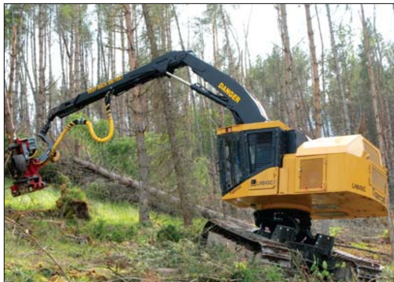
(Left) The 182HVT from Neuson-Ecotec works well in extremely difficult areas. (Right) Tigercat's LH845C, primarily designed for clearfell harvesting on slopes.
