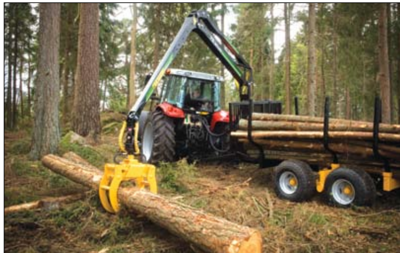
(Above) Mowi's Skog 85 eight-tonne trailer from Fuelwood is aimed at lighter forwarding and handling of pulp, firewood and smaller timber. (Below) Kesla offers a choice of 14 models, both drag and driven.
