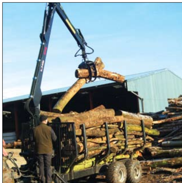
(Left) The Vreten range of trailers from Marshall Agricultural Engineering can handle loads ranging from 7-14 tonnes. (Right) The LMS/Palms range has trailers ranging from 8000-13000kgs, with cranes from 4.7 up to 8.4 metre reach.
