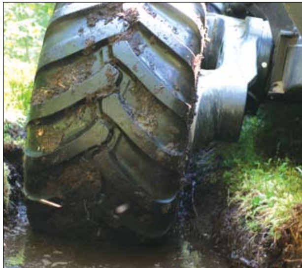
The large contact area on the Nokian Forest Rider radial tyre produces less surface pressure than that of a cross-ply forestry tyre.
