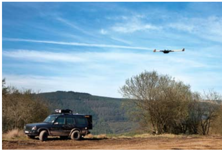
The G2 coming in to land near the ground station vehicle. Tracks or low vegetation make suitable operating sites.
