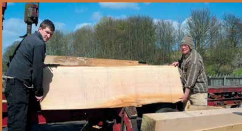
Neil and Dennis remove a high quality board which already shows the distinctive markings of quarter-sawn oak. The medullary rays that give rise to the pattern are cellular structures through which the living wood transmits preservatives to protect the heartwood from decay.
