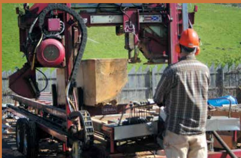
Dennis Anderson mills a couple of boards from one cut side of one of the quarters of the big butt. Prominent silver patterning will only be produced by a few cuts at this setting as the angle between the blade and the timber’s grain is gradually changing.
