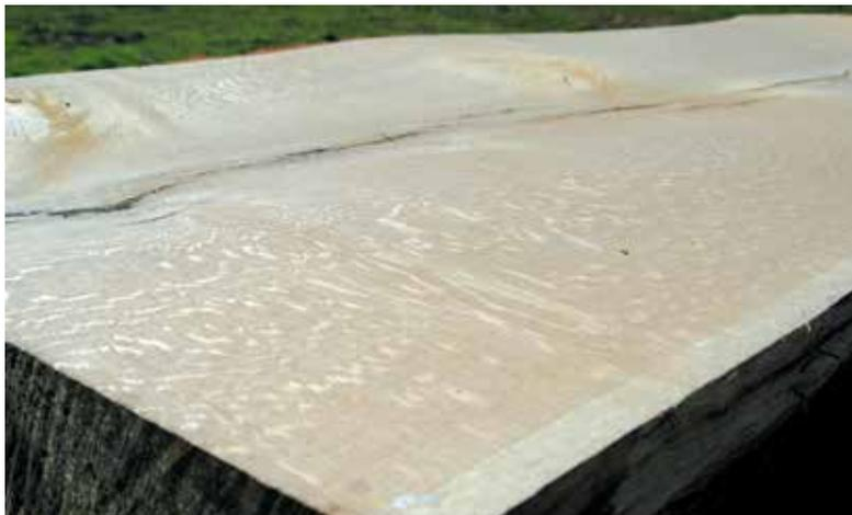
Two quarters of this oak butt are on their way to the sawbench. A chainsaw has been used to make the initial cuts and it has revealed the silver banding that Dennis is looking for.
