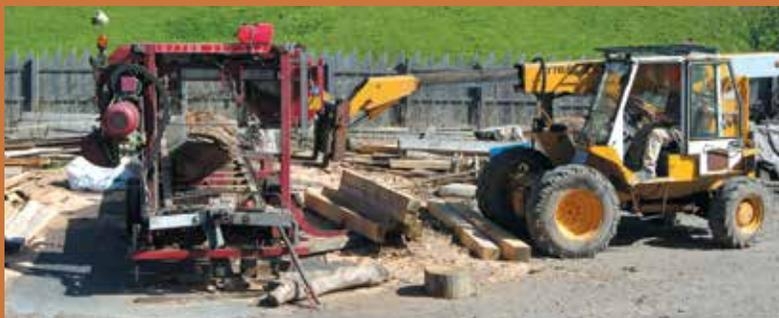
He has decided to turn the piece with the loader to take a few boards from the other flat side. It is a time consuming procedure that enables the maximum return of top quality boards with minimum waste.
