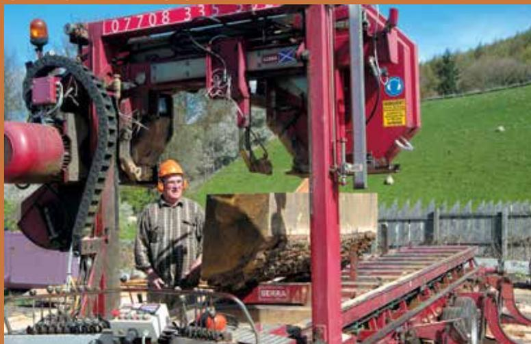
Dennis carefully considers whether he can take another board. The blade will have to cut more or less in the direction of the drying cracks that have appeared on the butt end to make the most of the timber’s properties.
