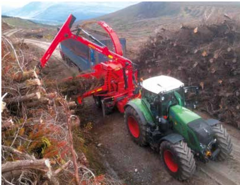
*The Eschlböck Biber 84 is a recent addition to the DGC Tree fleet and its performance has turned out to be more than satisfactory. The ability to load full sized road trailers in about 35–40 minutes will suit both the contractor and the haulier.*
