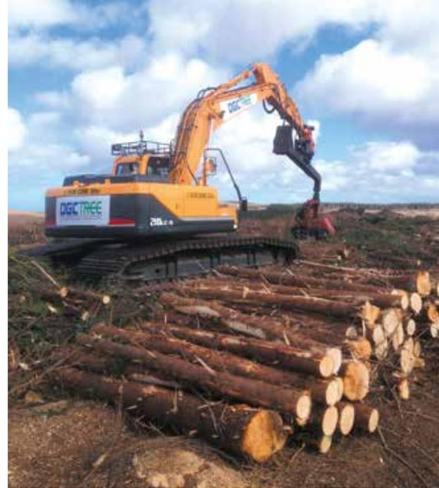
*For cut-to-length harvesting DGC Tree has opted for the Komatsu 370E harvesting head. Excavator bases fitted with wide pads for soft ground working need the support of the boom for efficient tracking – hence the special nose cone attachment designed by JCC and Drew Graham.*
