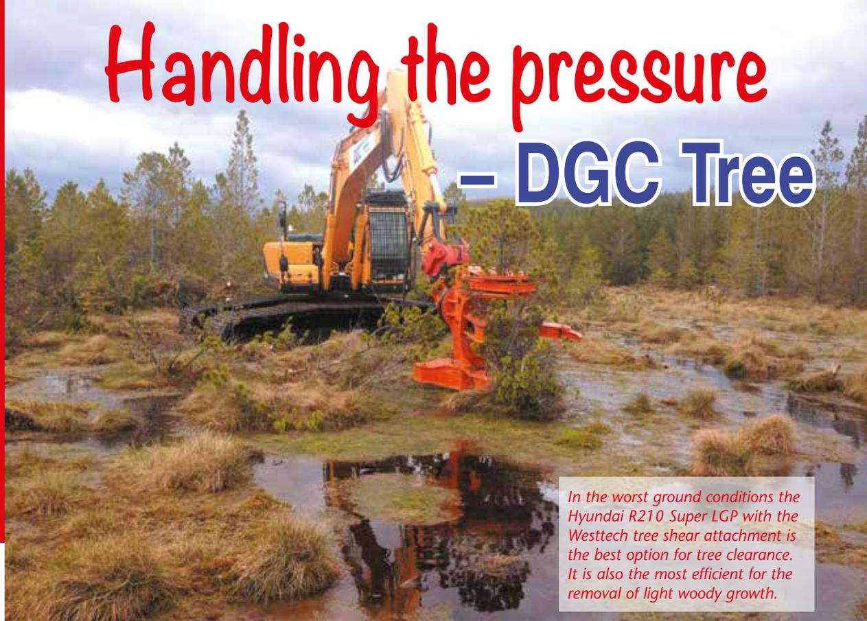
*In the worst ground conditions the Hyundai R210 Super LGP with the Westtech tree shear attachment is the best option for tree clearance. It is also the most efficient for the removal of light woody growth.*
