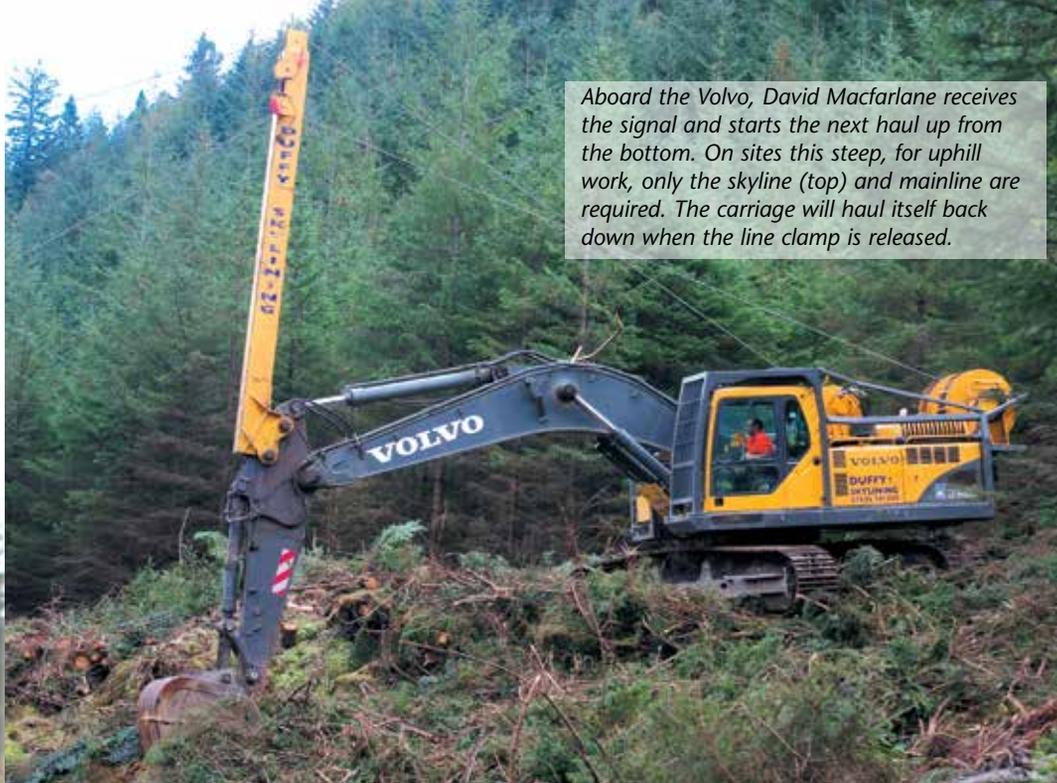
Aboard the Volvo, David Macfarlane receives the signal and starts the next haul up from the bottom. On sites this steep, for uphill work, only the skyline (top) and mainline are required. The carriage will haul itself back down when the line clamp is released.
