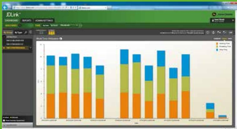
The JDLink 'work time utilisation' screen. This makes it possible to analyse how many hours a machine has been working and how effectively it has been operated.
