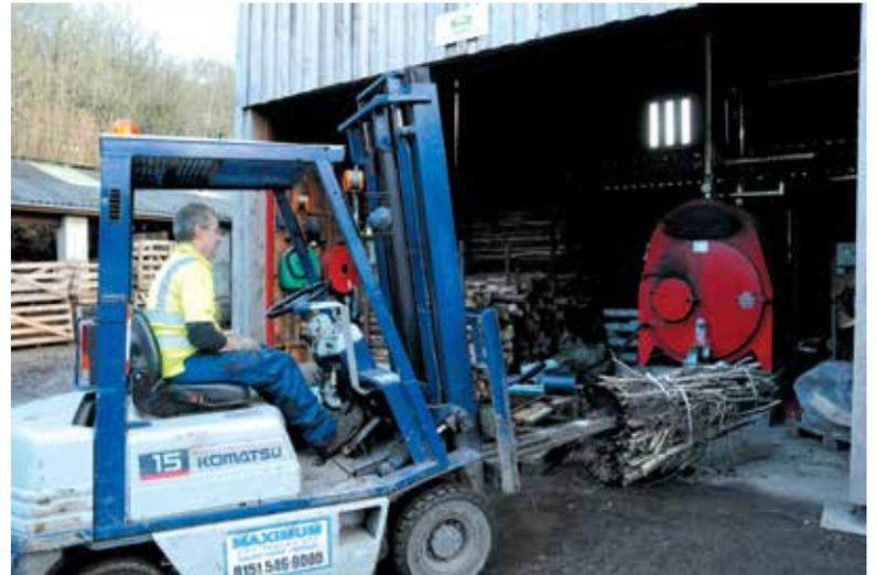
*Yard (and boiler) manager Ian Tredwell skewers a brush bale with a spike attachment on the Komatsu 15 forklift ready to feed the FARM2000 161kW biomass boiler.*
