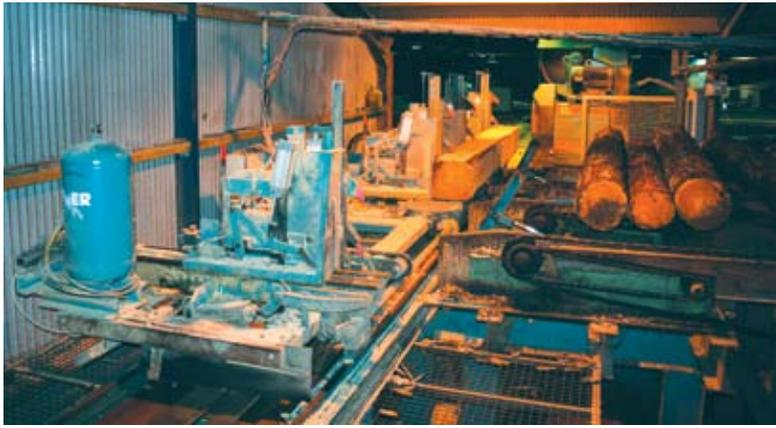
(Above) The log intake and carriage feeding the bandmill and LBL chipper in the large log line. (Below) The outfeed from the bandmill in the large log line.
