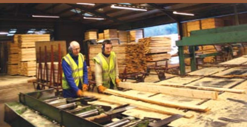
*Manual sorting of the finished boards in the small log line.*
