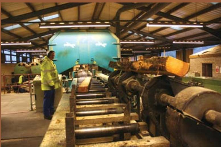
*The twin roller bed resaw in the small log line.*
