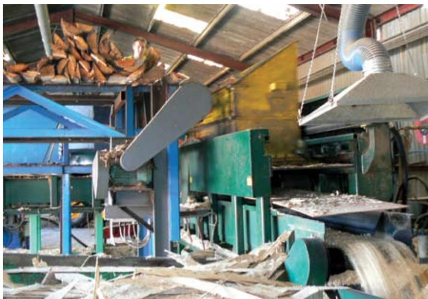
Cross-cutting with the Holtec saw.
