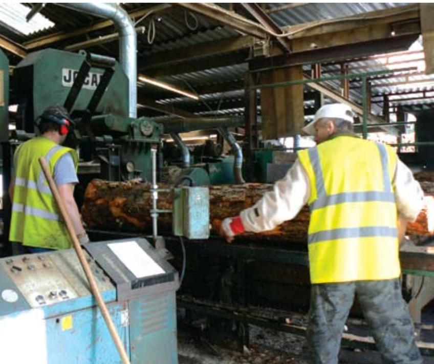
Eight-foot logs going through the Jocar twin saw at Llandrillo.
