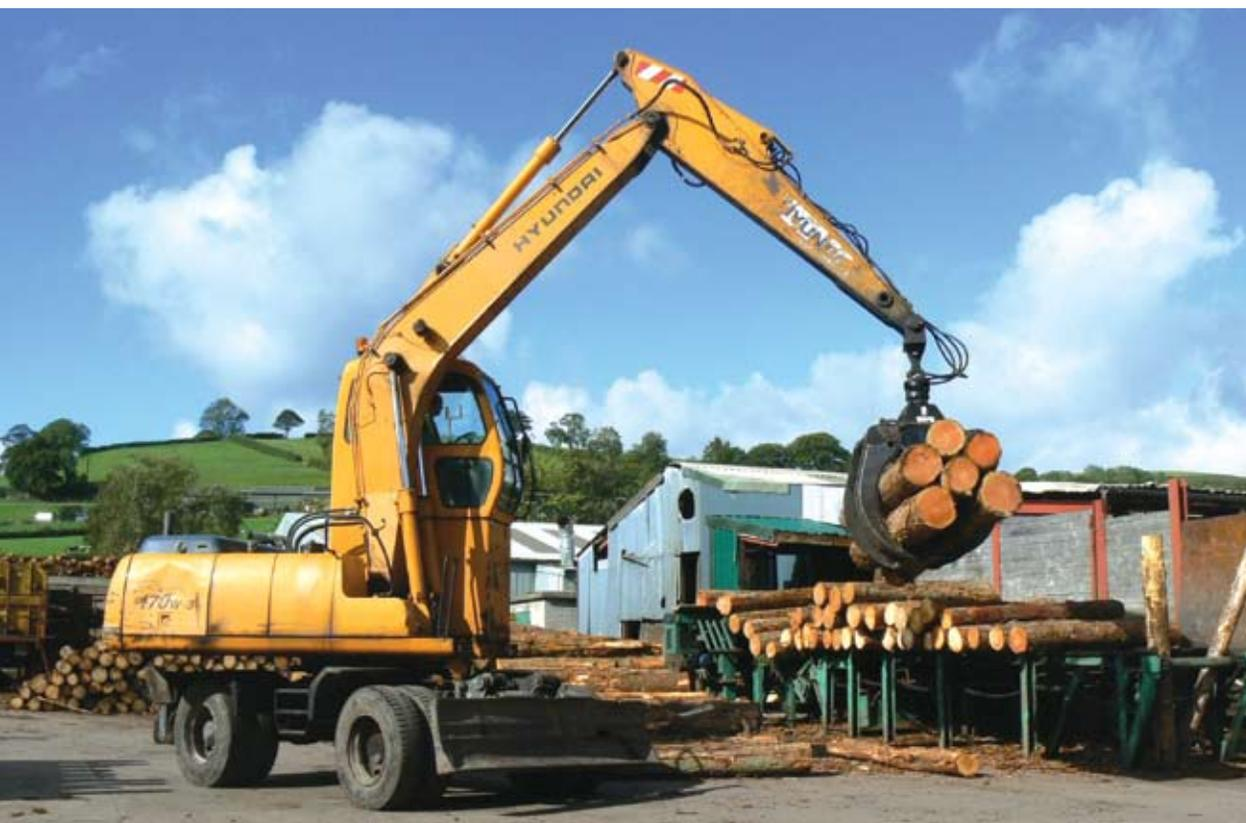
*The wheeled excavator loading eight-foot logs onto the log ramp in the old station yard at Landrillo.*
