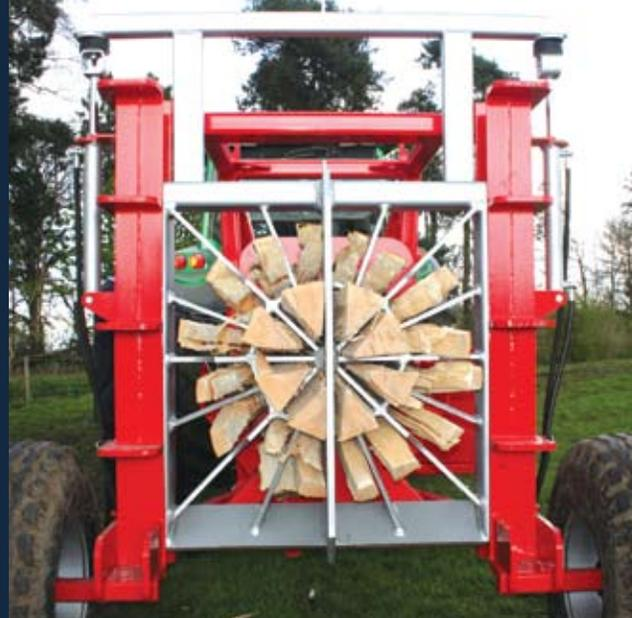
This 60-tonne splitter was sold to Nigel Cunliffe. Specifically designed for large, difficult timber, it will take logs up to half a metre in length, splitting them into 24 pieces.
