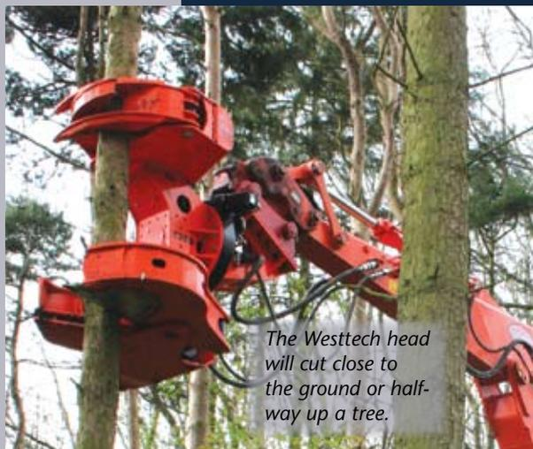
*The Westtech head will cut close to the ground or half-way up a tree.*
