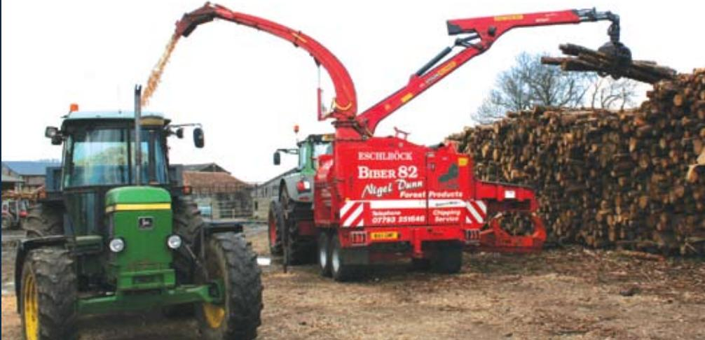
Joe Dunn demonstrated his Eschlböck Biber 82 chipper, powered by a Fendt 936 tractor. Over the two days the stack of logs was chipped ready for collection. Visitors to the demonstration commented on the excellent quality of the finished woodchips. Joe has a selection of different sized screens which are easily exchanged so he can produce chips of the size required by his clients. Any logs too big to fit through its 55x38cm feed opening are broken up using the attached Westtech L700 Woodcracker.
