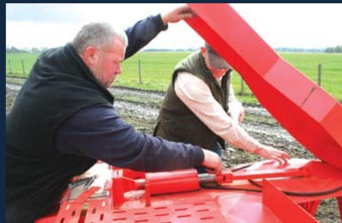
(Above) Simon is shown explaining the inner workings of the Woodpecker, a very simple device that makes kindling from old pallets and joinery waste.
