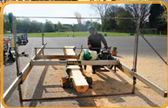
CEDAR FELLED IN SCHOOL PLAYGROUND, MILLED AND USED FOR RETAINING BORDER WHERE TREE ONCE STOOD.
