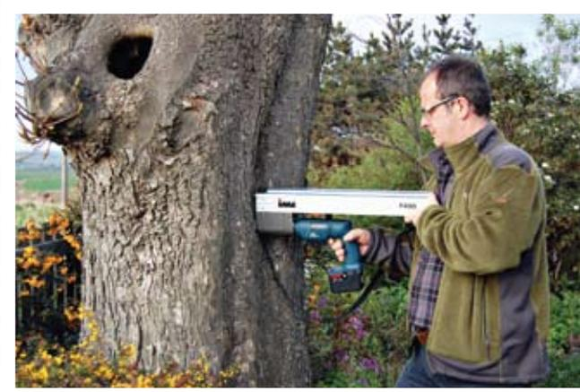
Testing the internal decaying of a tree using the Resistograph 400 decay detection device.
