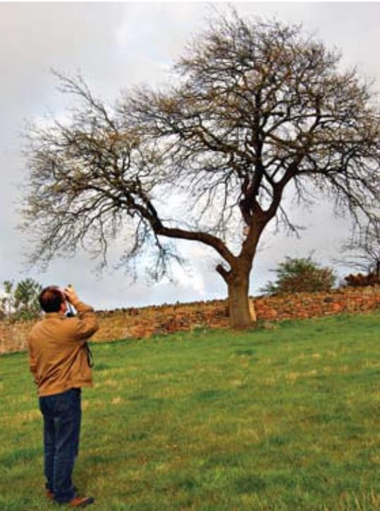
Measuring the height of a tree using the TruPulse Clinometer.
