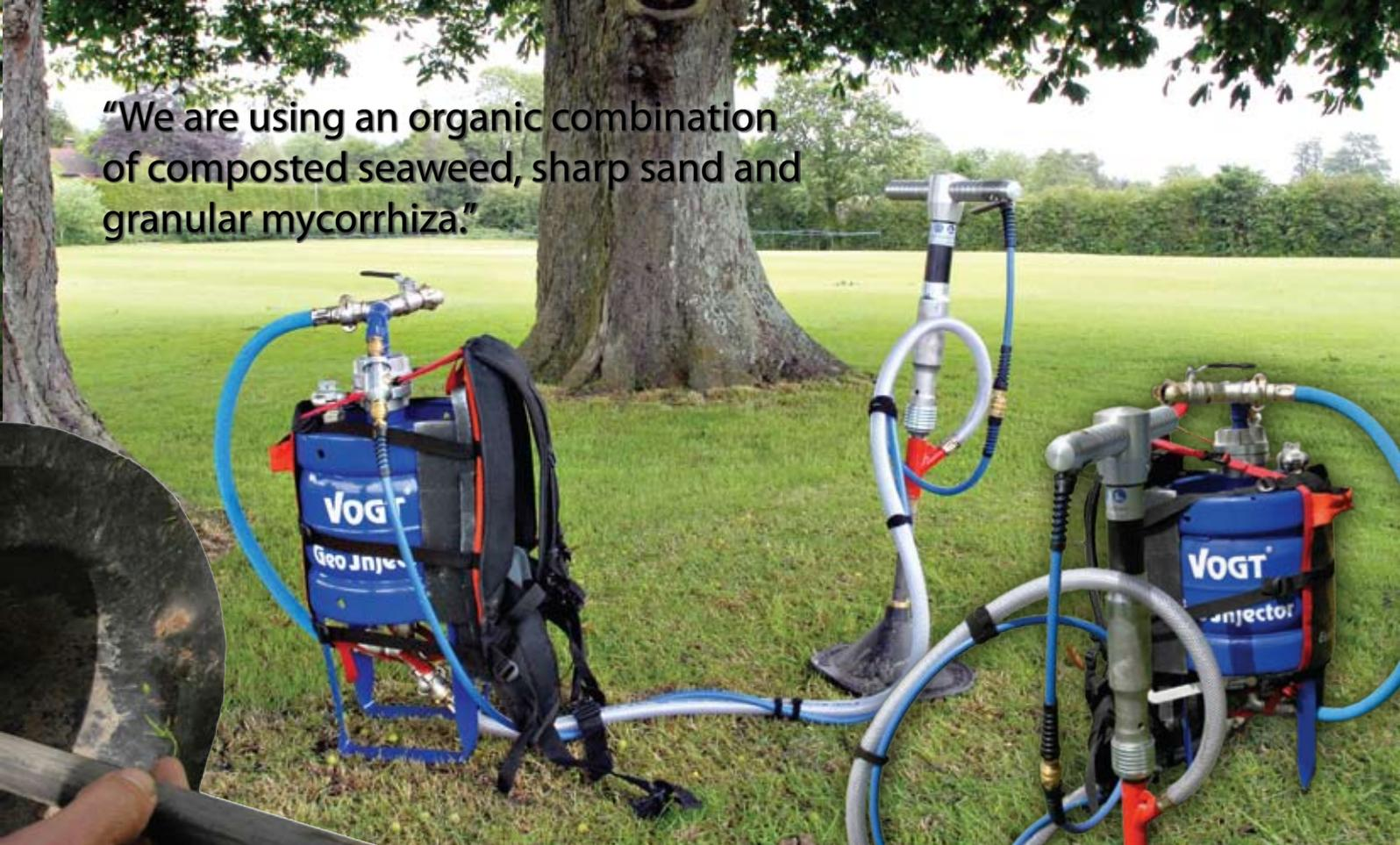
*The VOGT Geo Injector developed by VOGT in Germany.*
