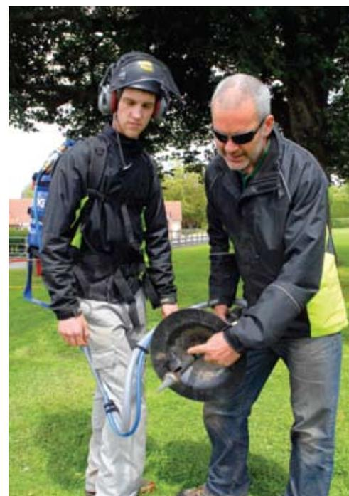
James stands while Matt shows that the drill is a metre-long spiked metal rod with hollow core. He points to the injector chutes – left and right.
