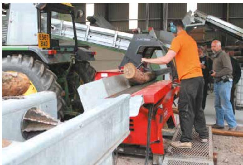
*The Dalen 2054 still has an important role to play in the processing yard, handling the smaller material. It is, according to the operator, a satisfying machine to work. Skill and experience can reduce to a minimum the inevitable splitting chamber blockages associated with the more simple processors. Power is supplied by a John Deere 2450 tractor.*
