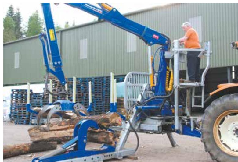
*The 6m bunk of the Binderberger forwarding trailer can carry two diameter selections from the stack to the firewood processors. The Binderberger L920 hydraulic splitter comes into its own reducing the largest diameter material alongside the trailer. The combination is extremely efficient for delivering to the processors from the stockpile, but also gives the option of working offsite.*
