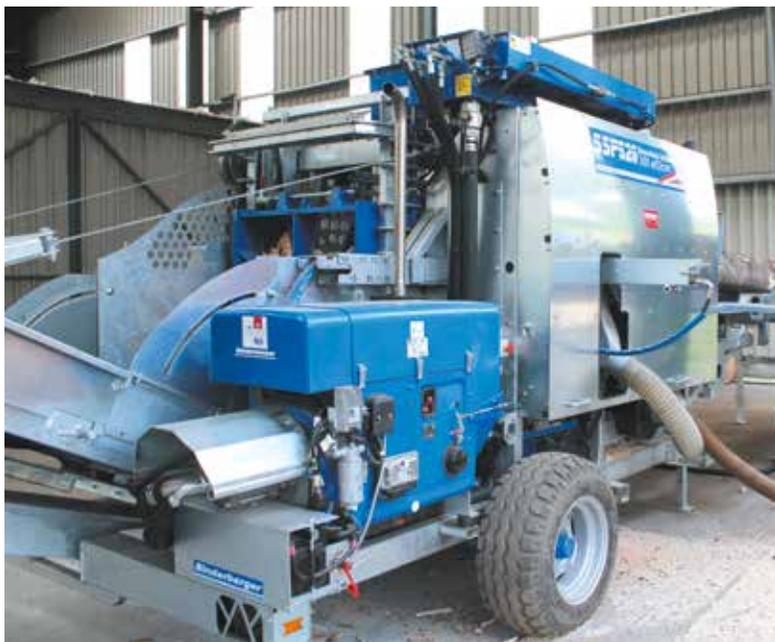
The new Binderberger SSP 520 is powered, like the Binderberger 450, by a Hatz Silent Pack diesel engine. Accepting material up to 52cm in diameter, the splitting force of 30 tonnes is applied to the sections as they meet the 16-way splitting knife. The output conveyor is suitably wide to conform with the machine's high output. The mobility of the two Binderberger processors eases the logistical problems of working offsite.
