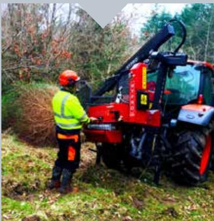
Smaller models in the range include the Hypro 300, with 35 m radio control winch and which can delimit trees up to 12"/30 cm. This machine has been in production since 1987 and they just keep going... there are 30-year-old examples still working hard all over England.
