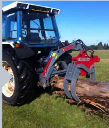
attach behind a tractor via the three-point linkage, onto a mini digger, or be mounted onto a front loader or telehandler via an adaptor plate. It also has the option of coming supplied with or without a rotator. These options increase the versatility of handling timber in a yard environment.
