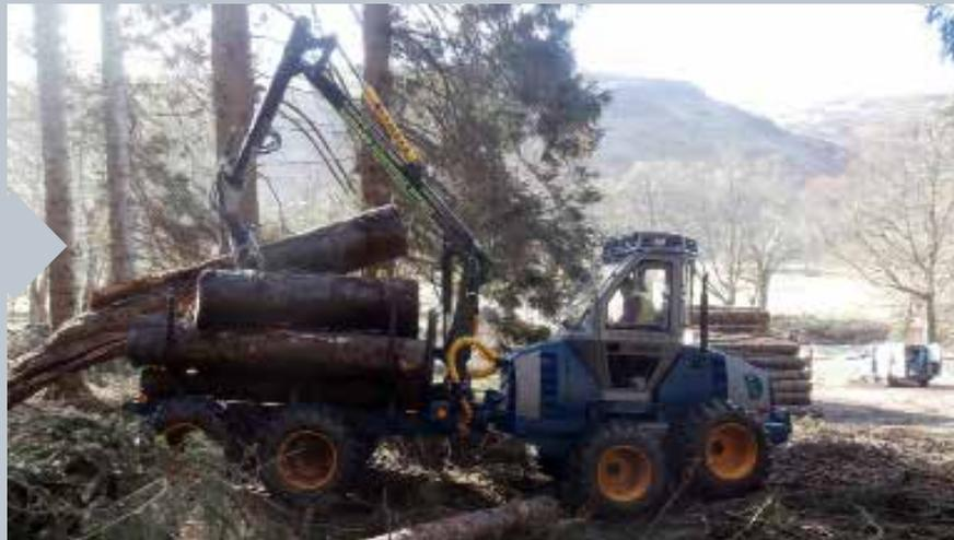
Slightly larger than the 511, the LVS 520 is also designed mainly for thinning. Like the 511, it features the sturdy 8-wheeled chassis, which, together with 500 mm tyres, provide good traction even in the most difficult forest terrains. The Cummins engine has a 60-kW output, with Sauer Danfoss hydraulic components, a SCAD control system from Adcis, and a Kesla
