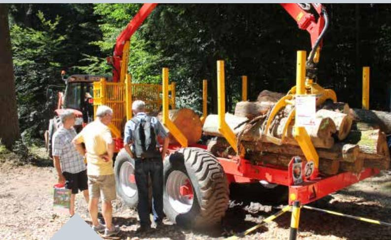
Rabaud's Xylotrail forwarding trailers (with capacities of 11 and 15 tonnes) feature a steering drawbar, but drive to the trailer wheels is not direct but merely 'assisted'. A hydraulic pump turns cage wheels between the tyres. Rabaud expects their customers only to require the extra traction occasionally.
