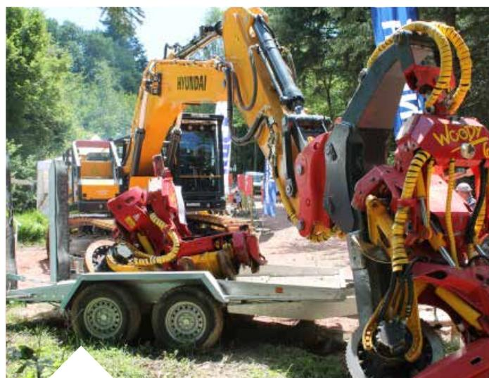
Olivier Saulnier works big timber in the Alps. For his latest machinery upgrade, Hyundai dealer Curty Materiels has supplied an HX 300NL excavator as a carrier for Olivier's Woody 60 harvesting head. Local Hardox steel fabricator Serrurerie Dunand was subcontracted by Curty Materiels to cut and fit the forestry protection that the contractor required for the rough ground he experienced in the mountains of Haute-Savoie.
