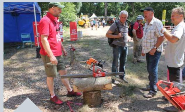
Irish-based chainsaw milling system producer Go2Mill took one of the small sites within the woodland circuit. The small chainsaw attachment runs on square-section timber or metal tubing and keeps the chain running true during the milling. Brian Gibson (left) and the Go2Mill team were very impressed with the reception their invention received and the sales produced.
