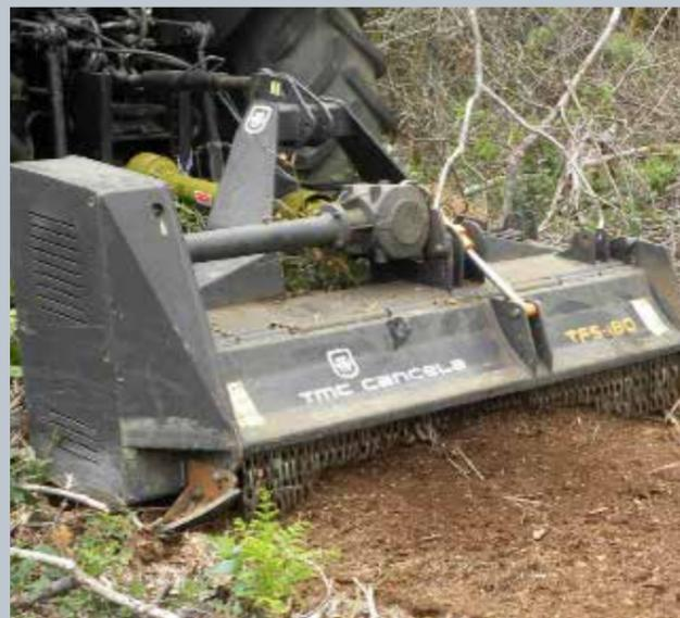
TMC's range of forestry mulchers benefit from bodies built with high-strength steel, avoiding cracks and breaks in the frames in the most demanding working conditions. Wear-resistant steel is used in those parts in contact with the ground, such as skates, plates, inner shells and counterblades, giving added durability.
