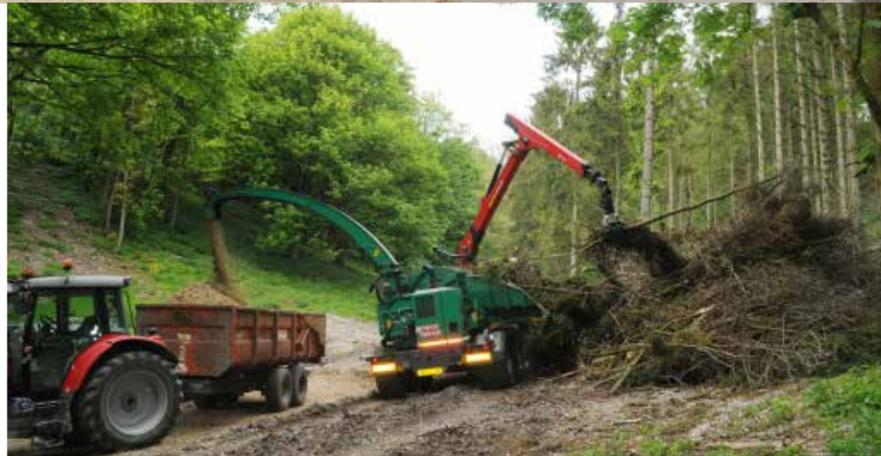
593Z chipper. With a 1.4 metre infeed, the machine utilises helix drum technology to chip, "giving a better sample when chipping brash (or a bushy tree)", at a rate of up to 40 tonnes per hour. Both are replacement machines bought last July. Vicary replaces most machinery every three years, before they get too worn.
