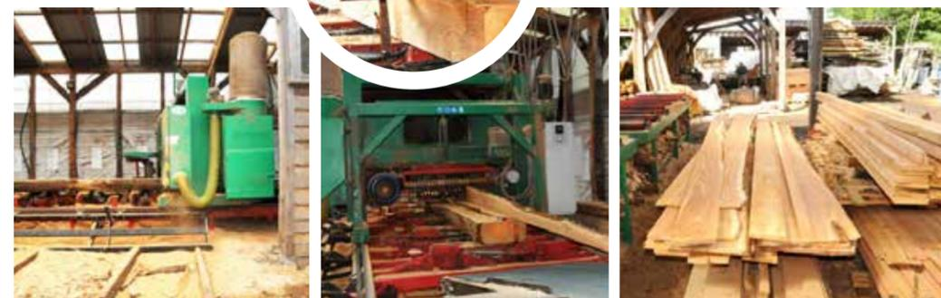
The Mebor HTZ1200 SuperProfi bandsaw's 24-foot log deck. Cutting Western red cedar for cladding, coming off with a waney edge (bark left on). All timber is manually loaded and manually removed.
