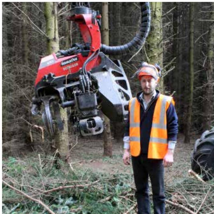
Simon Scott with the Komatsu C93 harvesting head. For the specialist thinnings contractor a neatly designed head that handles responsively through the standing crop speeds up the operation and avoids damage.
