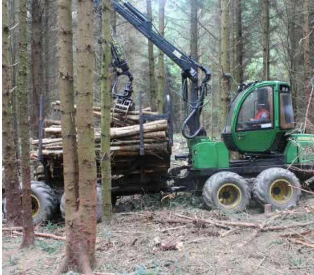
The John Deere 810E forwarder picks up timber destined for chipping and subsequent use in the estate's three biomass boilers. It is hard to justify loading poor-quality softwoods onto wagons and shifting it across the country when there is a profitable use on the doorstep.
