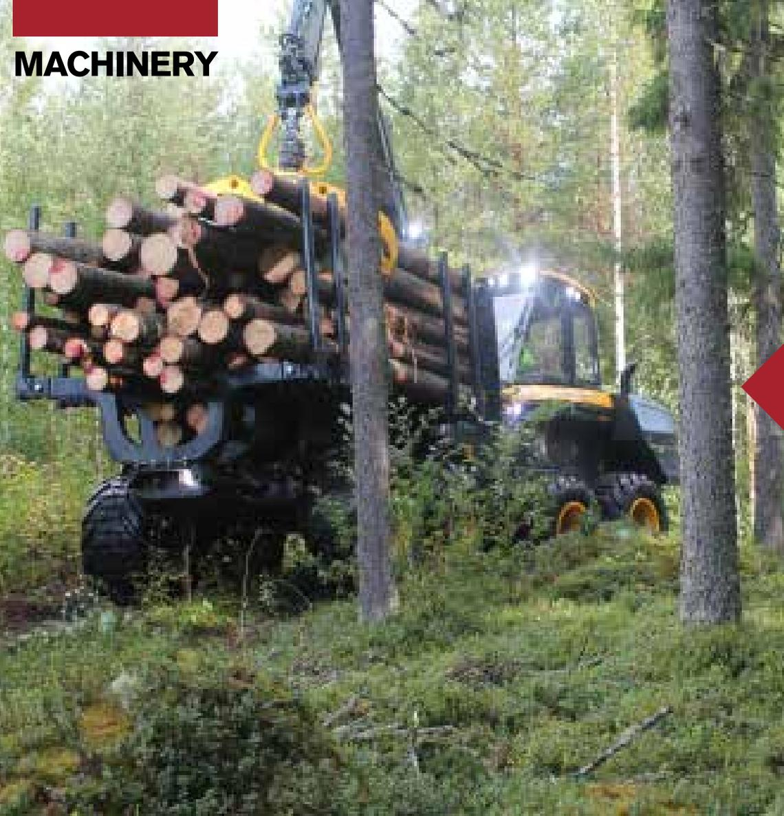
Left: The Ponsse Bison has a 16-tonne load capacity. The continuously variable transmission allows a stepless acceleration up to the top speed of 20 kph. The management system matches the load on the Mercedes Benz/MTU high-torque engine to the speed over the ground and optimises fuel consumption. Operator interventions, even on rough and difficult hauls, are reduced to a minimum.
