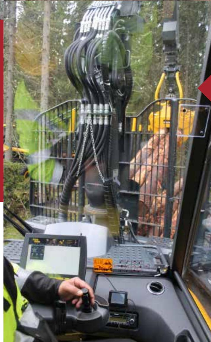
Above: The new Ponsse K121 loader has been designed for the Elephant and Elephant King forwarders. Increased lifting torque of 195 kNm and a slewing force of 48 kNm make the loader ideal for handling big timber on steep slopes. The generous grapple area of 0.5m<sup>2</sup> allows for big lifts both in the wood and at the roadside and speedy loading and unloading. Depending on the option chosen, the K121 has a reach of 8 m or 10 m.
