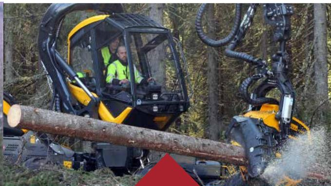
Above: The Ponsse Scorpion King is the harvester for difficult and challenging sites. While the Scorpion is equipped with a single hydraulic pump, the Scorpion King has a 145 cm<sup>3</sup> pump for the crane and a 190 cm<sup>3</sup> unit for the harvester head. The machine can be equipped with the H5, H6 or H7 harvesting head. For work in the eucalyptus forests the H7euca or the H77euca heads can be fitted.
