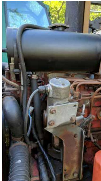
Stop solenoid with new wiring and miscellaneous diode removed now works faultlessly.
