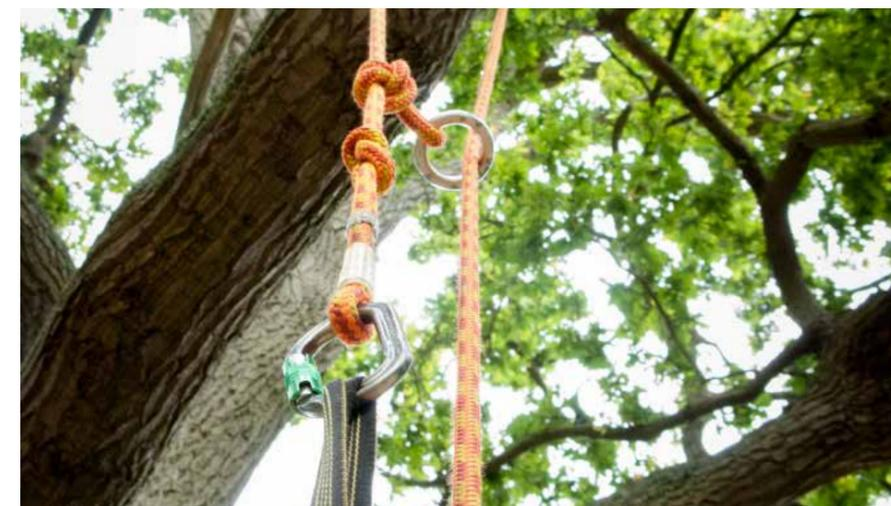
**I**N the last article we had a very brief look at canopy tie-offs when using an SRT system to access the canopy and, just to recap, one of the main advantages of using this system is that the load at the anchor point is equal to the weight of the climber (and equipment); unlike using the basal tie-off where it is effectively doubled.
